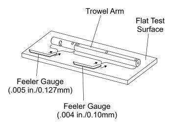
Figure 41. Checking Trowel Arm Flatness
